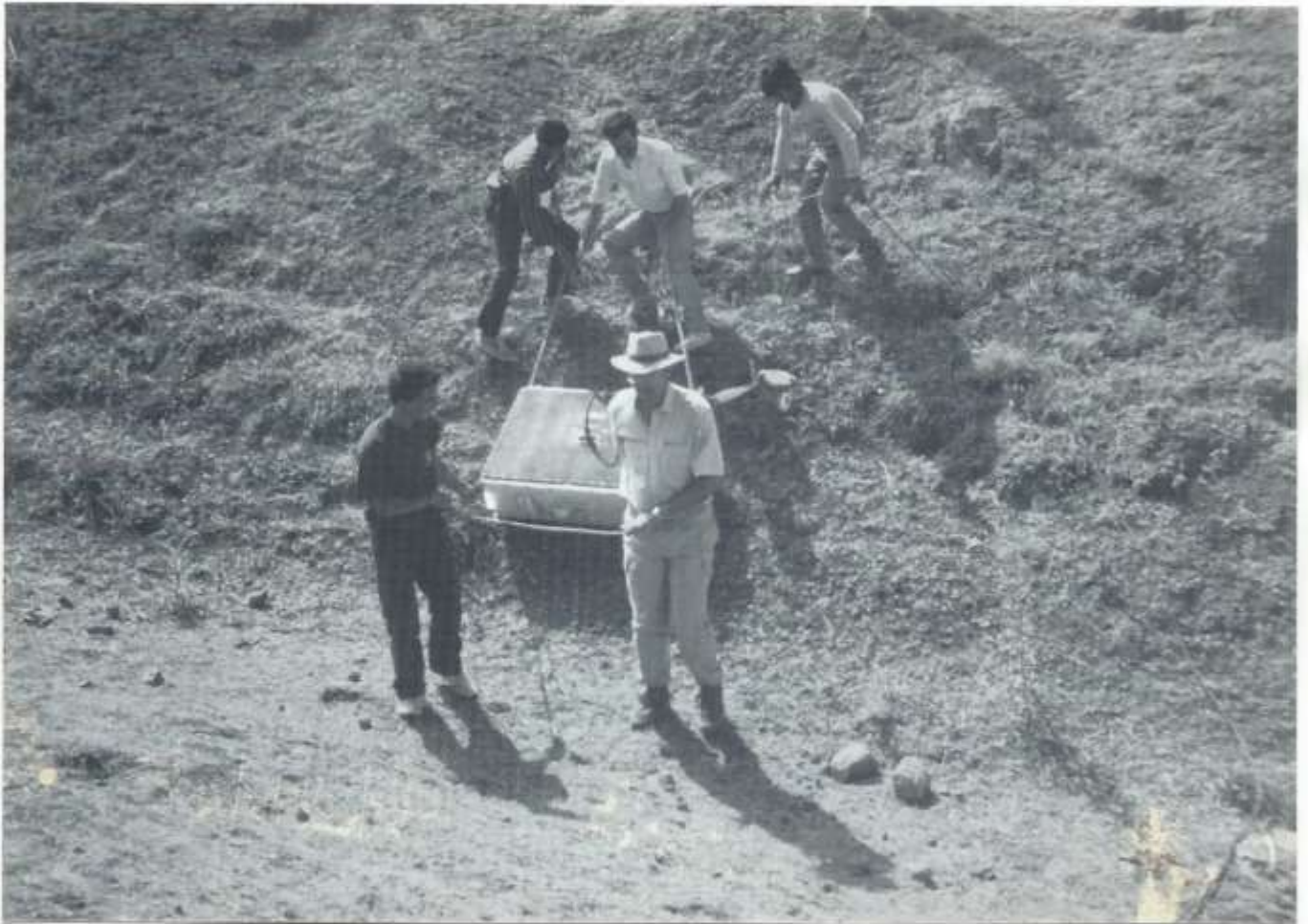
Fig. 5 Radar antenna is moved across the site at as uniform a speed as possible. Radar pulses 5 nanoseconds wide are transmitted 50,000 times per second. Energy reflected by the subsurface structure and received by the antenna is processed to provide a visual representation of the underground structure.
