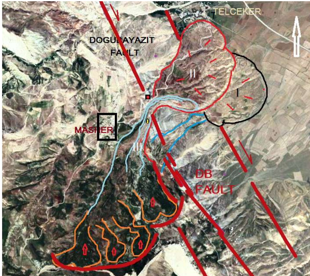
Figure 2. Telceker Landslide; Dogubayazit Faults and Three Stages of Debris Flows
